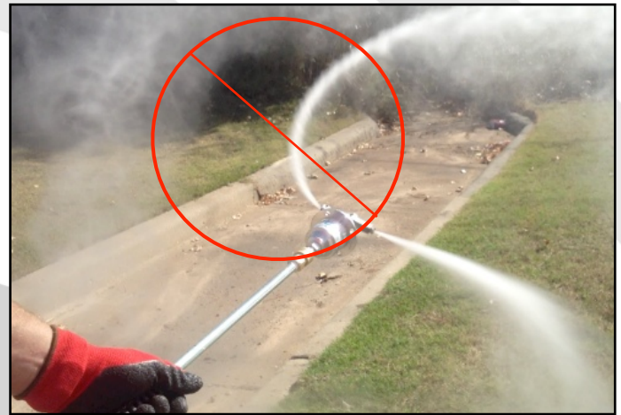
COMPETITORS HEAD RUNNING 3000 R.P.M. SPRAY REACH APPROX. 12" FROM SPRAY TIP
