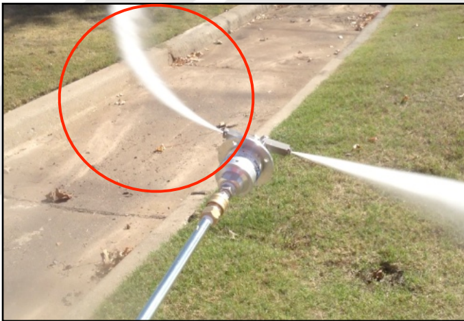
DRIPLOC HEAD RUNNING @300-500 R.P.M. SPRAY REACH
