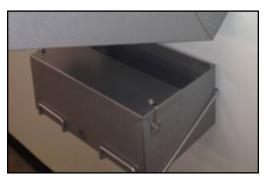
STEP #3 Finish by mounting Grease System as close do deflector pan as possible but allow lid removal
